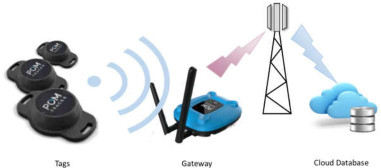
The system consists of tags that people carry, a gateway receiver that connects through a cell network to a cloud database.
