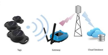
The system consists of tags that people carry, a gateway receiver that connects through a cell network or a tablet connection through the Internet to a cloud database.
